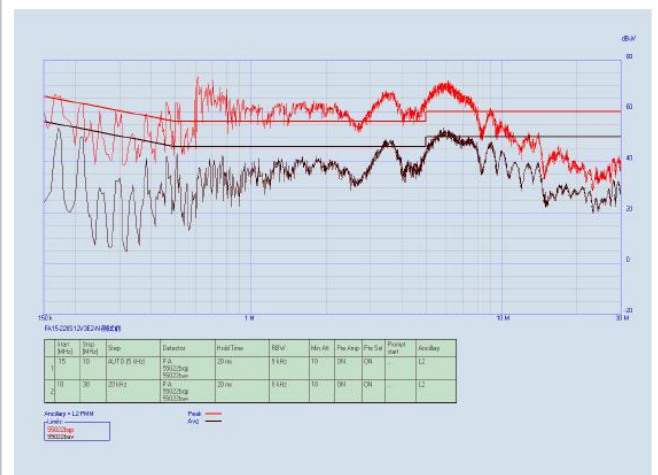
Input N line (no filter added) to test CE waveform
